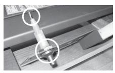
**21)** Plug up the Piezo hole with the plastic bushing.
